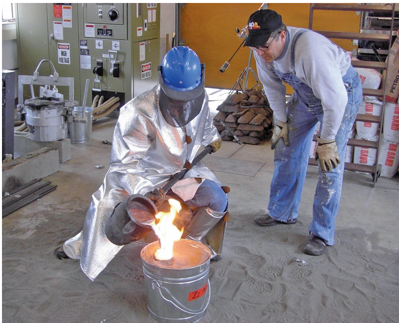
John (Chip) Keough supervises a student pouring molten aluminum in to a sand mold.
