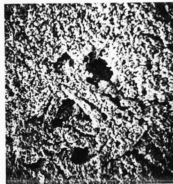
Fig. 10.32. Large voids formed by bridging of agglomerates in fine \text{Al}_2\text{O}_3 powder viewed with scanning electron microscope at 2000\times . Courtesy C. Greskovich.
