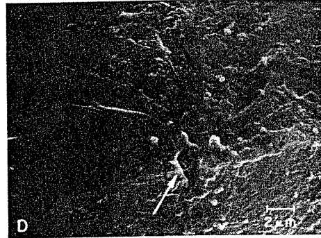
Fig 9 SEM fractographs of a fiber after removal of the metal coating. Source of failure (arrow) is from an elliptical defect, most likely from a bubble in the preform that was drawn out with the fiber.
