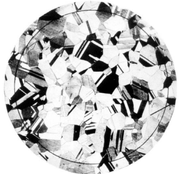
FIG. 3 Example of Twin Grains (Contrast Etch) from Plate III. Grain Size 0.090 mm at 75X
