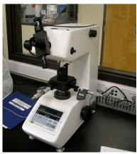
2. Turn on the instrument by pressing the "STANDBY" switch into the on position (do not touch the power switch)
