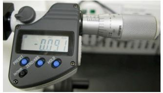
There are built in micrometers to make incremental adjustments in the position for both x and y directions.
