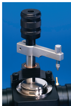
MIRacle High-Pressure Clamp – Ideal for Routine Sampling
