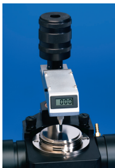
MIRacle Digital Clamp Ideal for Controlled Pressure
