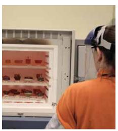
Oxidation-Reduction reactions are more fun when you apply them to make raku pots. Submerging the hot pot in a can with shredded newspaper reduces some of the metal oxides in the glaze, creating a unique metallic luster.
