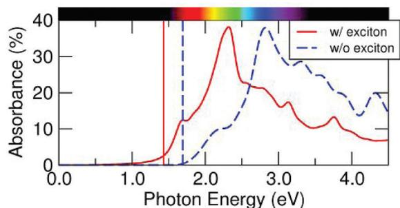
A SnSe monolayer has unusually strong absorbance in the visible range (up to 38%) and is a promising material for ultrathin photovoltaic applications. Image from G. Shi and E. Kioupakis, Anisotropic Spin Transport and Strong Visible-Light Absorbance in Few-Layer SnSe and GeSe. *Nano Letters* 15, 6926 (2015).
