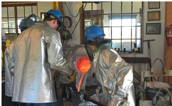
**At Keough's Joyworks Studio, MSE 360 students enjoy the work of transferring molten metal from the furnace, to the ladle, to be poured back into ingots.**
