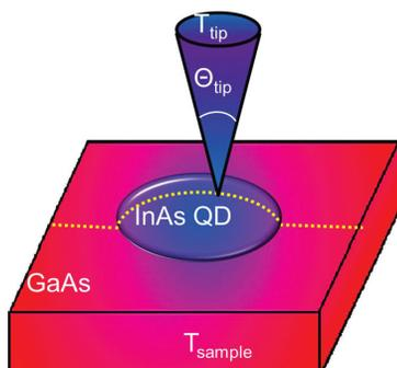
Schematic of the scanning thermoelectric microscope setup, which consists of a room-temperature probe tip in contact with a heated sample. The yellow dashed line represents the measurement points of the thermoelectric voltage at each tip-sample contact.
