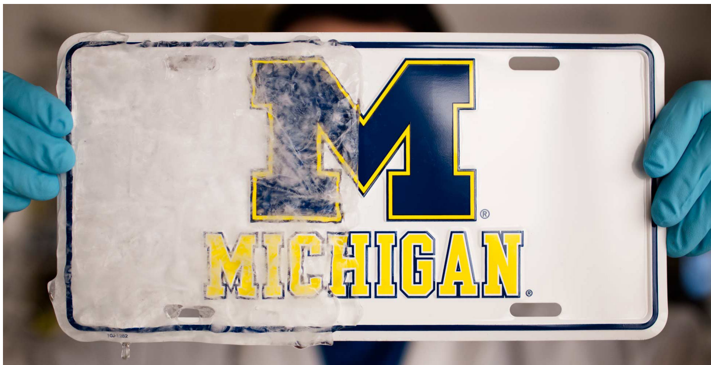
Fig. 1 - Icy conditions applied to a license plate – the left side is uncoated; the right side is coated with new icephobic substance being researched by Anish Tuteja's group.
