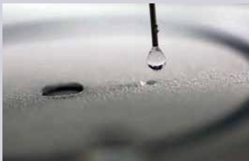
Mathew Boban, Macromolecular Science & Engineering PhD student, and Kevin Golovin, MSE PhD student, test a superhydrophobic surface by burning it as part of its resistance testing against water.
