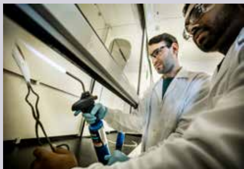
Mathew Boban, Macromolecular Science & Engineering PhD student, and Kevin Golovin, MSE PhD student, test a superhydrophobic surface by burning it as part of its resistance testing against water.
