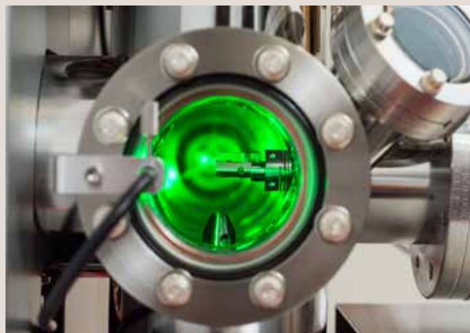
(MC) 2 upgraded its atom probe tomography instrument with a new Cameca LEAP 5000HR.
