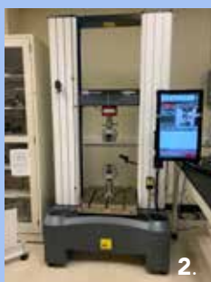
New equipment in the Van Vlack Lab: 1. A new HaasVF-1 five-axis CNC machine. 2. A new Instron 3382A load frame for mechanical testing. 3. An Objet24 stereolithography 3d printer.
