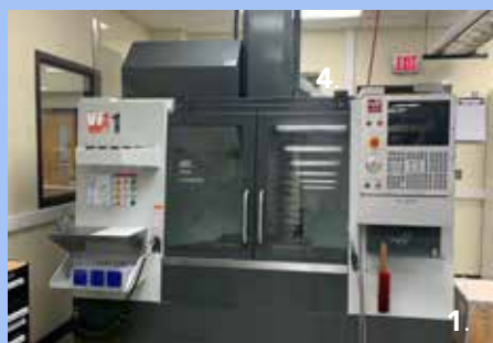
New equipment in the Van Vlack Lab: 1. A new HaasVF-1 five-axis CNC machine. 2. A new Instron 3382A load frame for mechanical testing. 3. An Objet24 stereolithography 3d printer.
