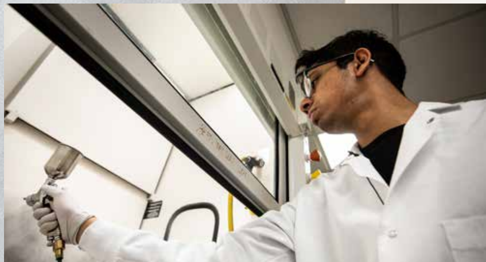
Abhishek Dhyani, Macromolecular Science & Engineering Ph.D. student, sprays a low interfacial toughness (LIT) coating onto a surface. The coatings help shed ice effortlessly from large surfaces and could be used on cargo ships, airplanes, power lines, wind turbines, oil rigs, and commercial buildings.
