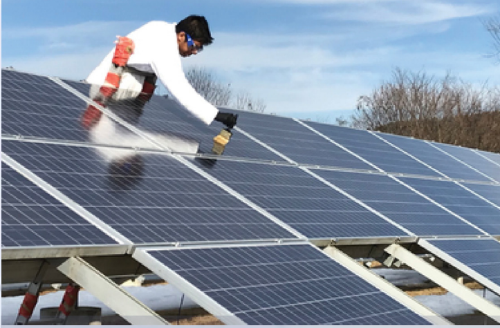
U-M macromolecular science and engineering graduate researcher Abhishek Dhyani applies ice-and-snow-repellent coating to a solar panel in Fairbanks, Alaska. Credit: Laurie Burnham, Sandia National Laboratory
