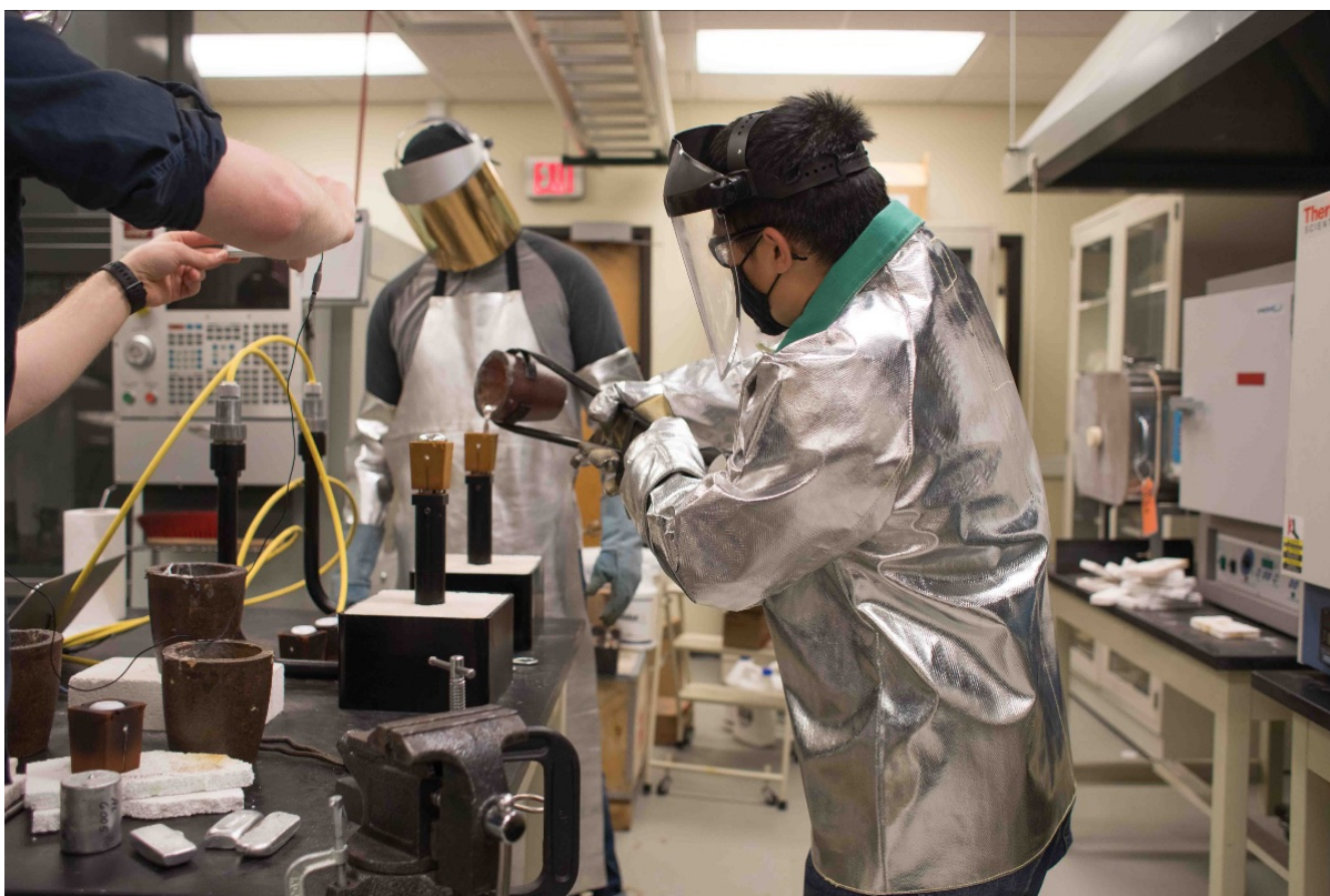
Paul Chao pours liquid aluminum into a crucible to measure its temperature as it solidifies.
