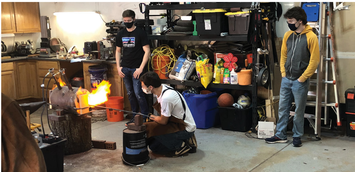
Grant Saxman heats the billet to be used in the hydraulic press afterward as Jeff Tschirhart and Alex Shaw look on.
