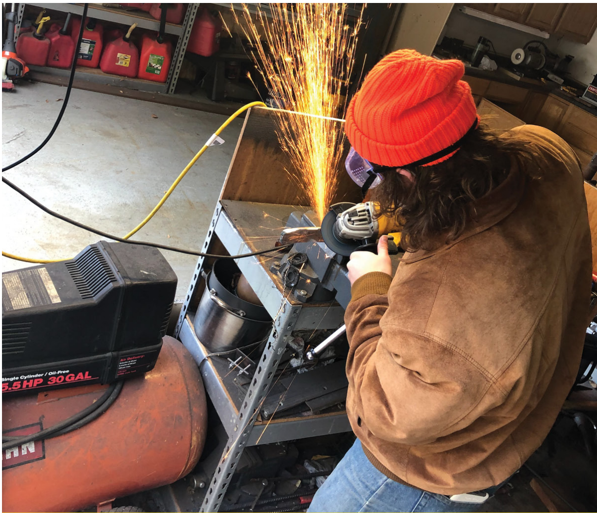
Jack Eilers uses the angle grinder to remove scale off the billet.
